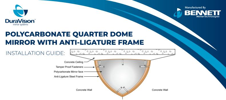
NOTE: If installing with Rawl Spikes, it is recommended to use a punch. This is to eliminate damage to the mirror and powder-coated frame.
